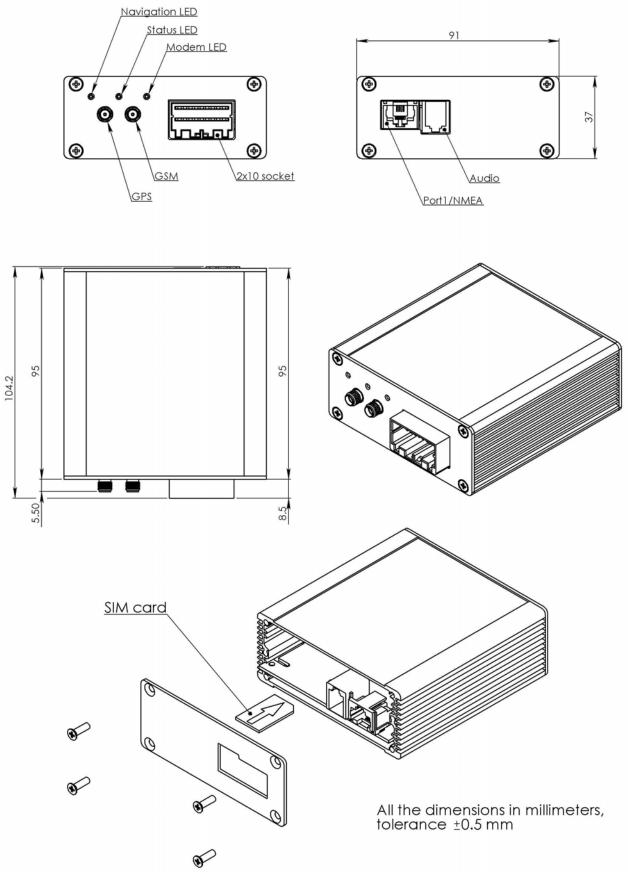
Figure 1. FM4100 drawing & spec, two enclosures
