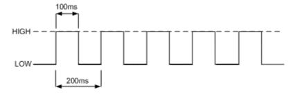
When GPS signal is received, the **Navigation LED** is blinking as follows:
