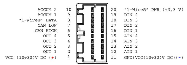
Figure 2. 2×10 socket pinout
