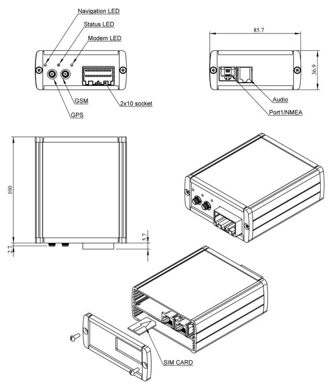
All the dimensions in millimeters, tolerance  $\pm$  0.5 mm
