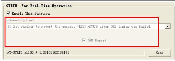
Choice F is used to set whether to report the message +RESP:GTGSM after fixing was failed.
