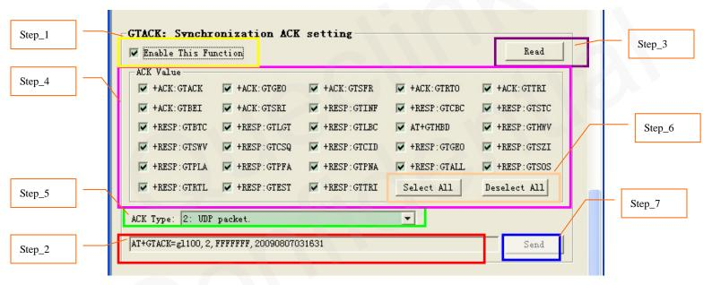
The purpose of Synchronization ACK function is to provide a way to make sure the message from GL100 to backend server was sent successfully. Please refer to "GL100 @Track Air Interface Protocol" for detail.
