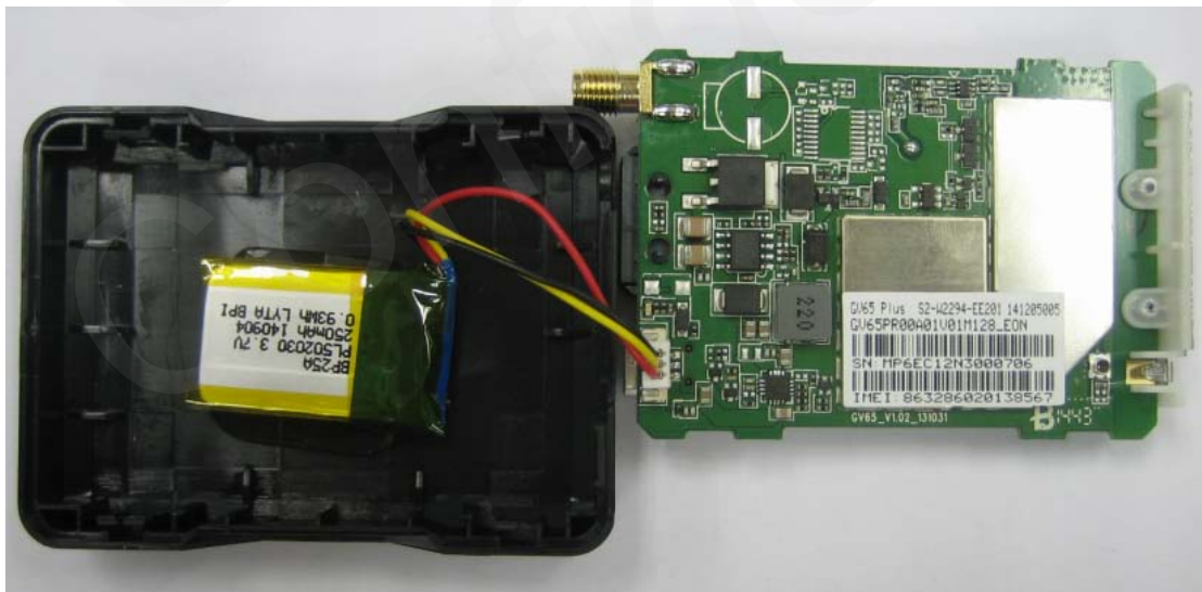
Figure 6. Internal Backup Battery
