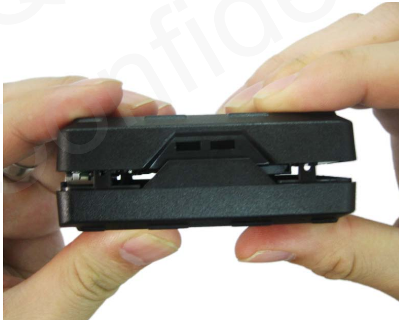
Figure 4. Closing the Case
