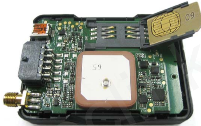
Figure 5. SIM Card Installation
