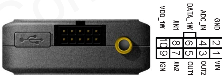
Figure 2. The 10 PIN connector on the GV65Lite
