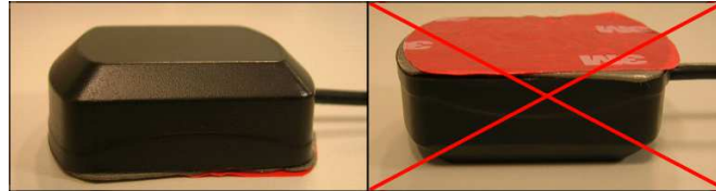
Figure 60 Correct GNSS antenna mounting
